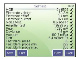
**HGB** measured impulses per second Measuring **Electrode voltage**, **current** and **offset**.
